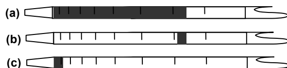
Fig. 5 Color Reaction of 141L a) Normal, b) Cucumber gas, c) Air at 100% humidity
